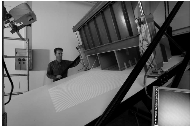
Fig. 2 View on the sluice gate and the reservoir at the channel inlet.
