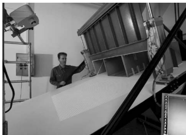
Fig. 2 View on the sluice gate and the reservoir at the channel inlet
