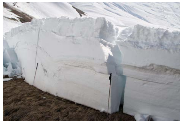
Figure 2. Part of the slab came to a halt after a short slide. The ski pole (135 cm) gives an indication of the snow depth. Photograph taken in the starting zone, on the far right of the upper crack seen in Fig. 1.
