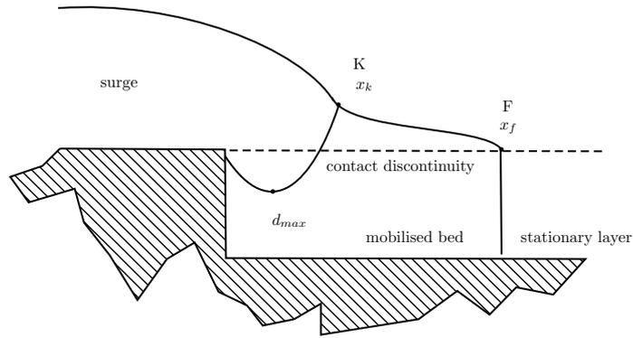
Figure 4: A material surface, called the “contact discontinuity”, separates the surge from the bed material. Experimentally, this interface can be tracked by using fluids of different colours. The front (point F) is the point of furthest reach, at which the flow depth drops to zero. The intersection of the contact discontinuity and free surfaces is represented by point K (where the flow depth profile displays a kink).
