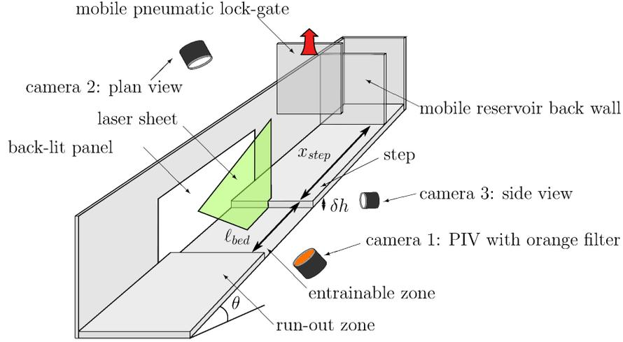
Figure 3: Experimental set-up including reservoir, lock-gate, step and bed, as well as the location of the laser sheet. The flume was tilted at slope angle  $\theta$  and the bed dimensions were  $\ell_{bed}$  long by  $\delta h$  deep.
