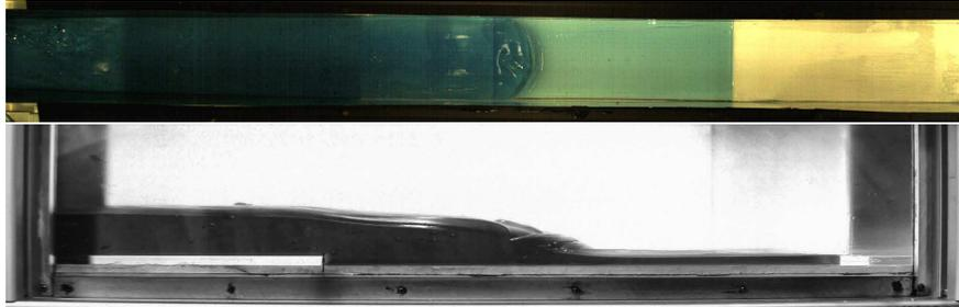
Figure 6: Images from camera 2 (top) and camera 3 (bottom). Camera 2 took plan views of the flow during entrainment, whereas camera 3 took side views. Combined experiment 20-6Ca, at  $20^\circ$  with entrainable bed dimensions of 6 mm deep by 30 cm long.
