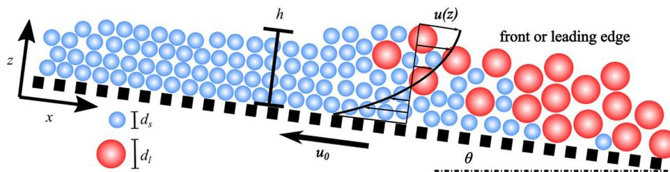
**Fig. 1** Sketch for the theoretical framework of the conveyor belt flow configuration. A stationary avalanche flows over an inclined moving plane forming a front or leading edge. For bidisperse avalanches, this
