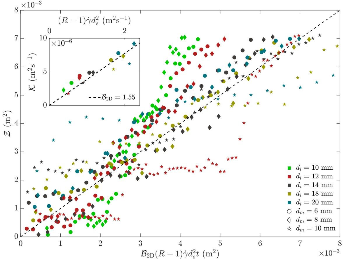
FIG. 3. All the intruder trajectories collapsed onto the identity dashed line given by the parametrized depth  $\mathcal{Z}$  and time  $\mathcal{B}_{2D}(R-1)\dot{\gamma}d_s^2t$ . The inset plot shows the fitted constants  $\mathcal{K}$  for each experiment as a function of  $(R-1)\dot{\gamma}d_s^2$ . The dashed line in the inset plot has a slope of  $\mathcal{B}_{2D} = 1.55$  and it is determined by a linear regression of  $\mathcal{K}$  as a function of  $(R-1)\dot{\gamma}d_s^2$ .
