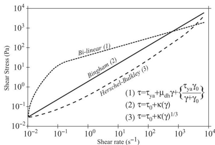
**Figure 1.** Typical flow curves of the three rheological models implemented in *BING*.
