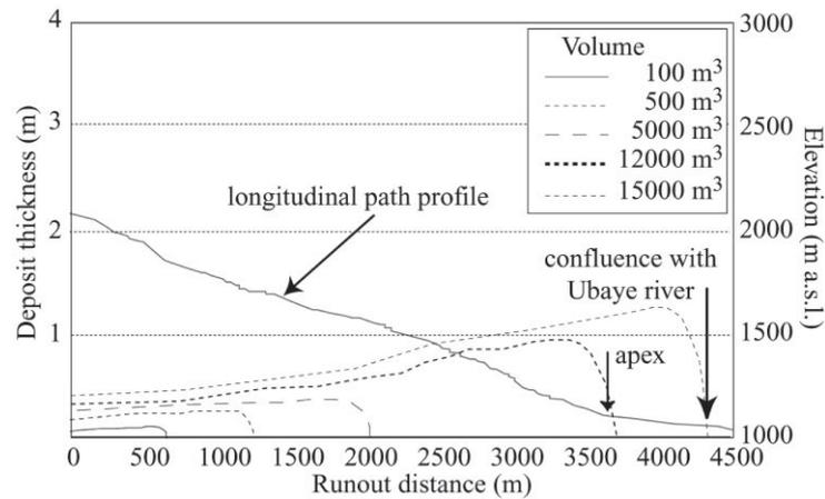
**Figure 6.** Estimation of the debris volume necessary to reach the apex of the torrent and the Ubaye River confluence for LTFI (for  $\phi = 0.45$ ).
