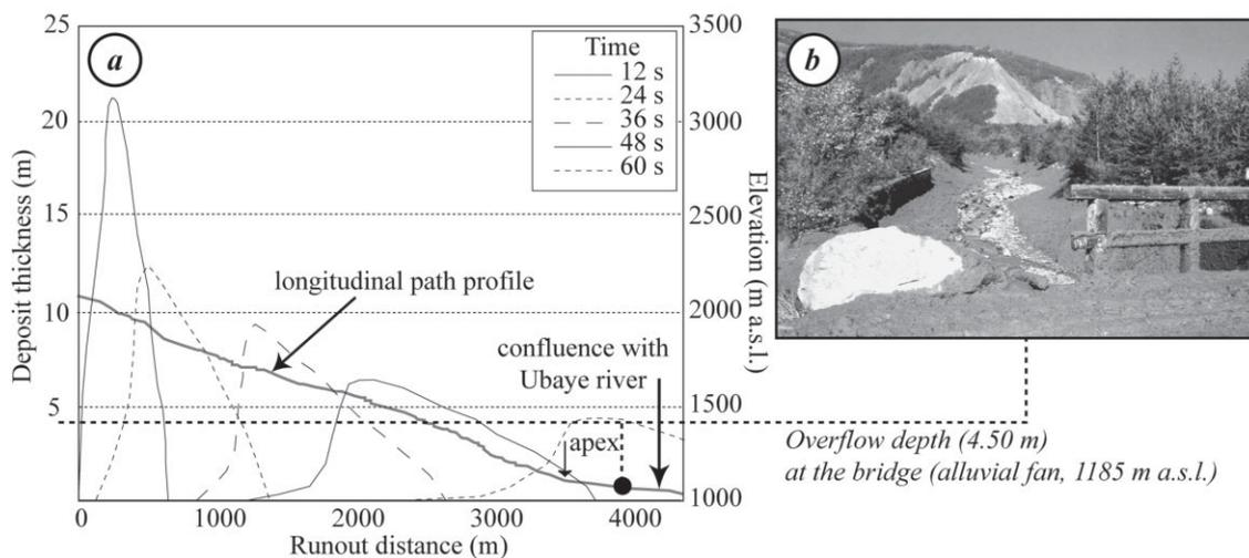
Figure 5. Computed debris-flow geometry overflowing at the apex (a) and photograph of the 1996 debris flow overflowing at the bridge (b).
