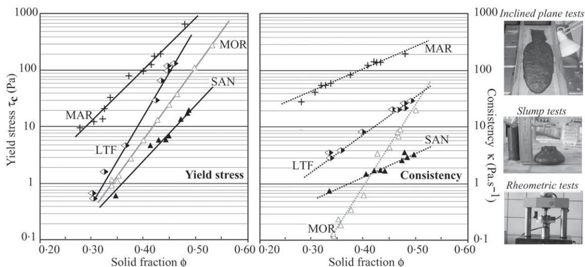
**Figure 2.** Herschel-Bulkley rheological model characteristics (yield stress and consistency) of the debris-flow deposit (LTF) and for the three main surficial deposits as a function of the total solid fraction ( $\phi$ ).
