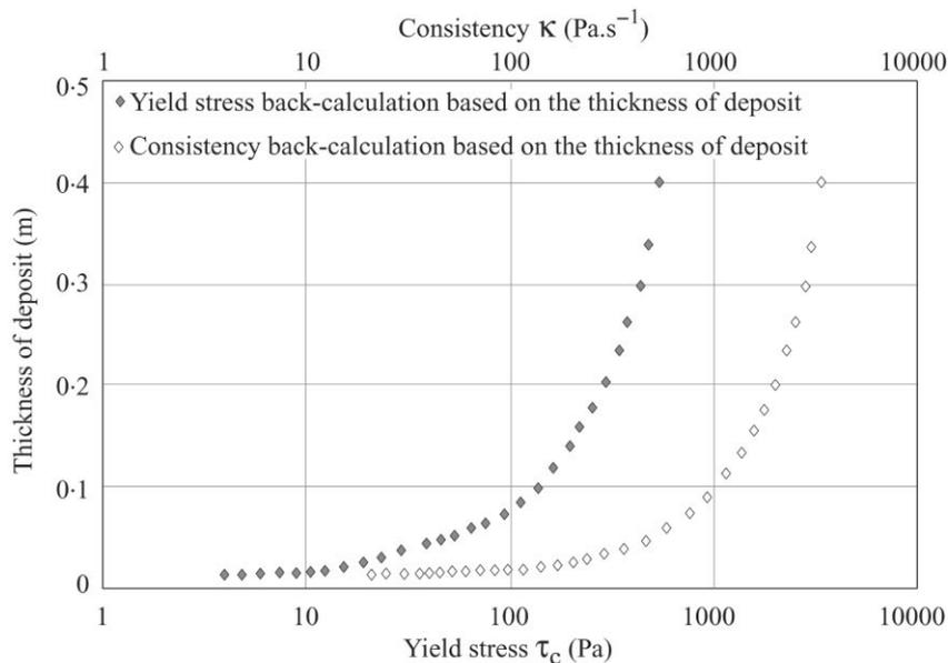
Figure 4. Data plots showing debris thickness as a function of material yield stress and consistency.
