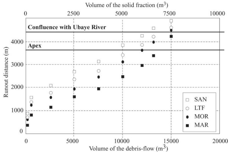
**Figure 7.** Relationship between the debris-flow volume and the runout distance for the three main surficial deposits and the 1996 debris-flow material.
