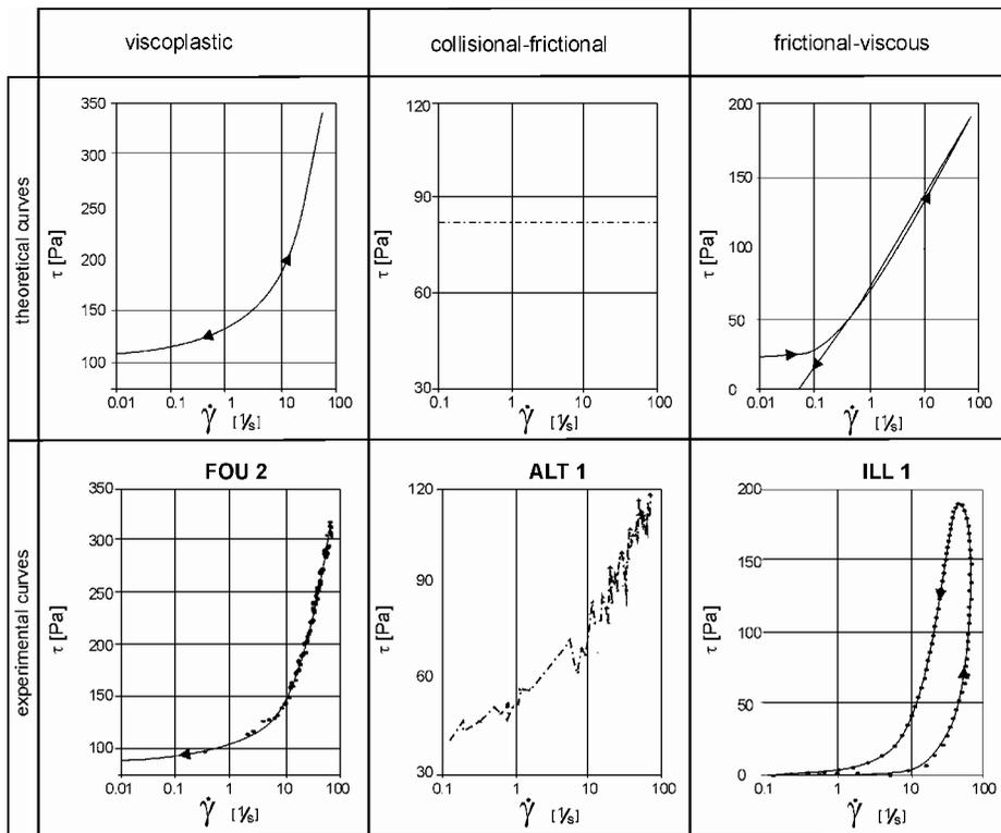
Figure 6. Comparison between theoretical curve and experimental rheograms obtained for some representative watersheds.
