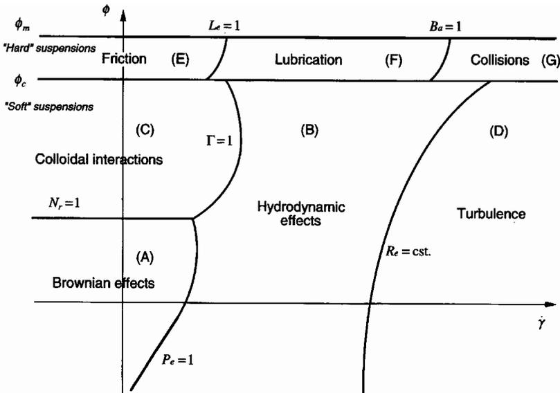
Figure 1. Simplified diagram of flow regimes, where  $Pe$  = Péclet number,  $Nr$  = repulsion number,  $\Gamma$  = a ratio between viscous and colloidal interactions,  $Re$  = Reynolds number,  $Le$  = Leighton number,  $Ba$  = Bagnold number,  $\phi_m$  = the maximum random solid concentration and  $\phi_c$  = the minimum concentration for a network of particles in close contact to form (for more details see Coussot & Ancey 1999).
