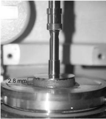
Figure 4. The rheometer used in this study, note the 2.8 mm gap between both plates.
