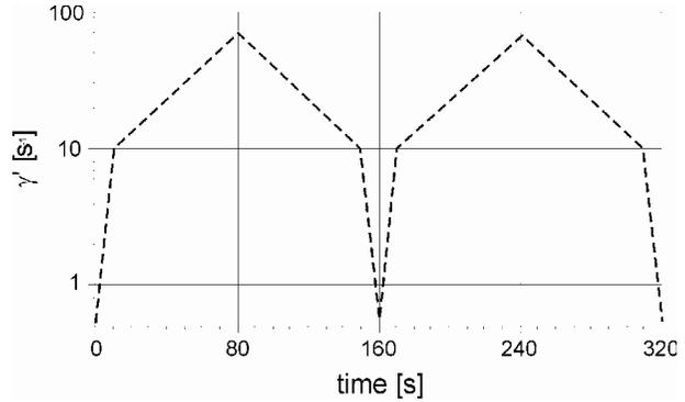
Figure 5. Rotating conditions procedure during the rheometric tests.
