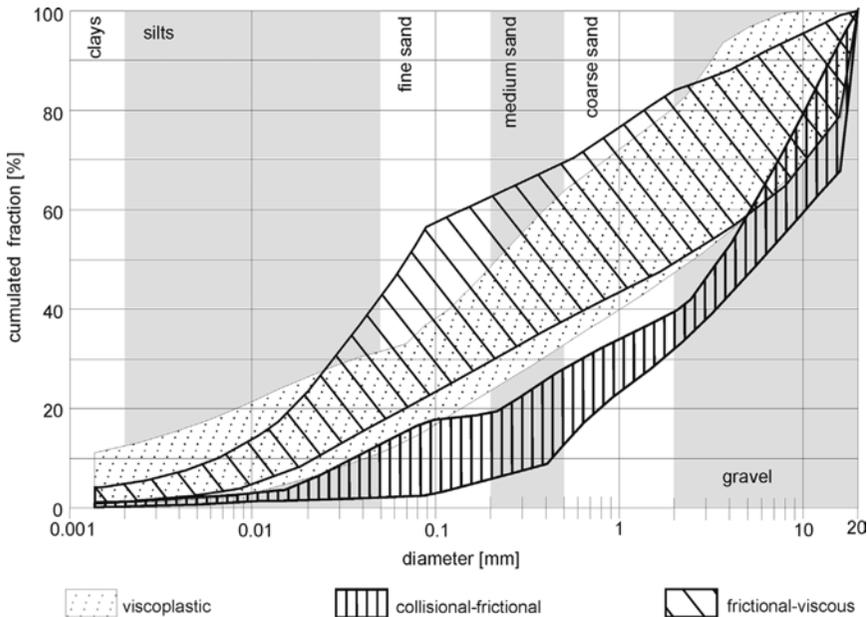
Figure 8. Envelope of grading curves of every samples of debris flow deposits, plotted with indication of their mechanical behavior.
