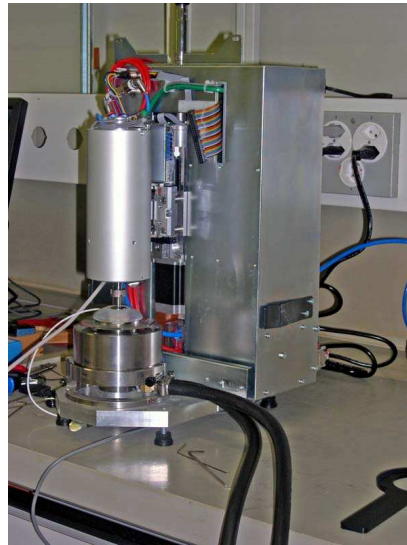
Figure 5.2. Bohlin CVOR used at LHE.
