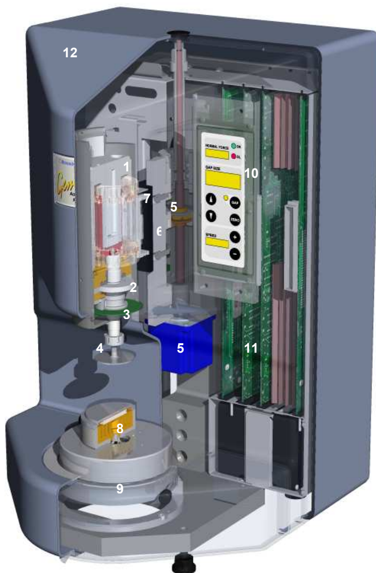
Figure 5.3. Bohlin CVOR used at LHE.
