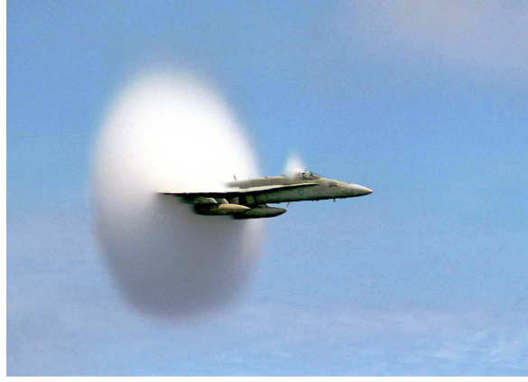
Figure 1.8. A U.S. Navy airplane creates a shock wave as it breaks the sound barrier. The shock wave is visible as a large cloud of condensation formed by the cooling of the air. A smaller shock wave can be seen forming on top of the canopy.(U.S. Navy photo by John Gay).
