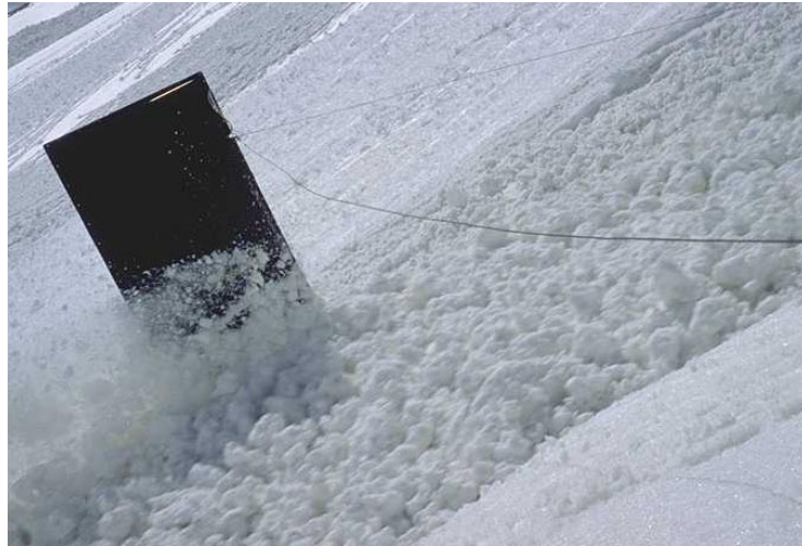
Fig. 2. Flowing avalanche impacting a wing-shaped structure in the Lauratet experimental site (France)
