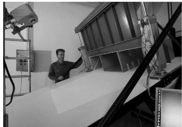
**Fig. 2** View on the sluice gate and the reservoir at the channel inlet
