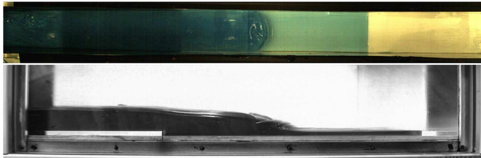
**Fig. 6.** Images from camera 2 (top) and camera 3 (bottom). Camera 2 took plan views of the flow during entrainment, whereas camera 3 took side views. Combined experiment 20-6Ca, at  $20^\circ$  with entrainable bed dimensions of 6 mm deep by 30 cm long.
