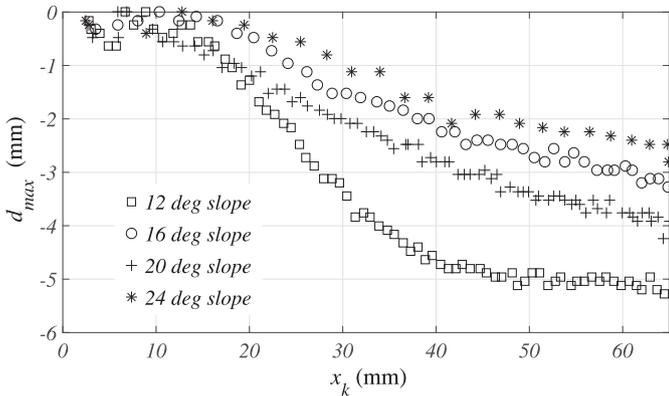
**Fig. 17.** Variation in the maximum interface depth  $d_{\max}$  with kink point  $x_k$ . For  $\theta = 12^\circ$  and  $16^\circ$ , the entrainable bed was located at  $x_{\text{step}} = 70$  cm, whereas for  $\theta = 20^\circ$  and  $24^\circ$ , the bed was located at  $x_{\text{step}} = 90$  cm.
