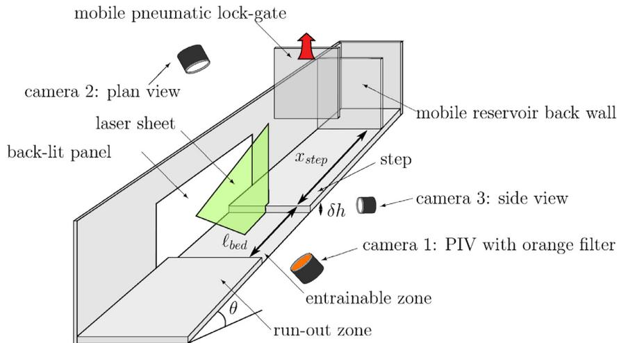
**Fig. 3.** Experimental set-up including reservoir, lock-gate, step and bed, as well as the location of the laser sheet. The flume was tilted at slope angle  $\theta$  and the bed dimensions were  $\ell_{bed}$  long by  $\delta h$  deep.
