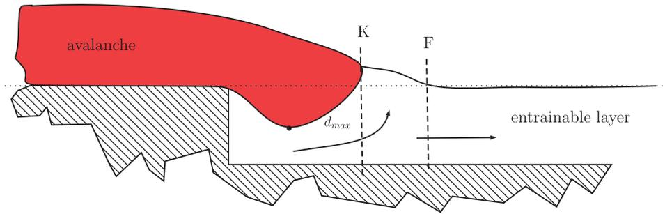
**Fig. 19.** Diagram showing the bed deformation caused by the incoming surge. Point  $K$  corresponds to the intersection between the contact discontinuity and the free surface: the furthest downstream point with fluid from the reservoir at that moment. Point  $F$  corresponds to the flow front, i.e. the furthest point downstream with  $h(x, t) > 0$ . The maximum excavation depth  $d_{max}$  is also shown.
