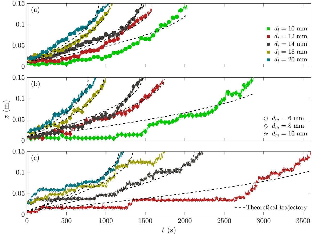
FIG. 2. Vertical position  $z$  as a function of time  $t$  for the intruders of  $d_i = 10, 12, 14, 18$  and  $20$  mm (in colors, see legend in (a)) segregating through the (a)  $d_s = 6$  mm ( $\bullet$ ), (b)  $8$  mm ( $\blacklozenge$ ), and (c)  $10$  mm ( $\star$ ) medium. The dashed lines ( $---$ ) plot the theoretical fits (see Eq. (6)) to the experimental trajectories, all of which used a value of  $\mathcal{C} = 0.271$  and  $\Phi = 0.7$ .
