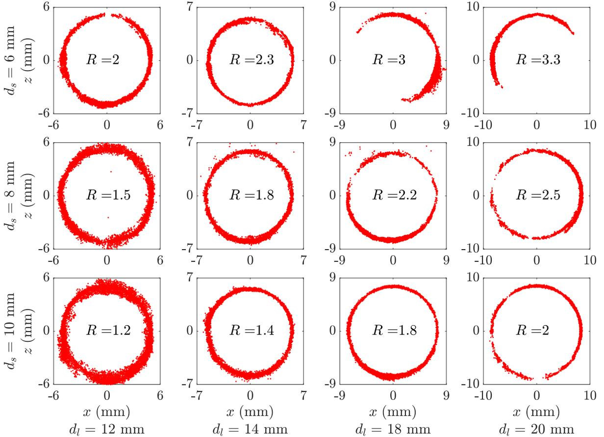
FIG. 4. Dot positions relative to the intruder’s position. Top row (left to right): experiments using a  $d_s = 6$  mm medium, with  $d_l = 12, 14, 18$  and  $20$  mm intruders. Middle row (left to right): experiments using a  $d_s = 8$  mm medium, with  $d_l = 12, 14, 18$  and  $20$  mm intruders. Bottom row (left to right): experiments using a  $d_s = 10$  mm medium, with  $d_l = 12, 14, 18$  and  $20$  mm intruders.
