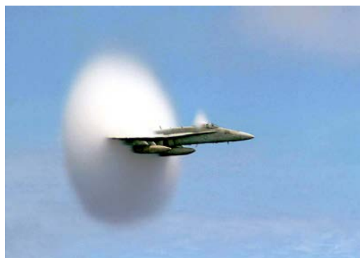
Figure 1.8: A U.S. Navy airplane creates a shock wave as it breaks the sound barrier. The shock wave is visible as a large cloud of condensation formed by the cooling of the air. A smaller shock wave can be seen forming on top of the canopy.(U.S. Navy photo by John Gay).
