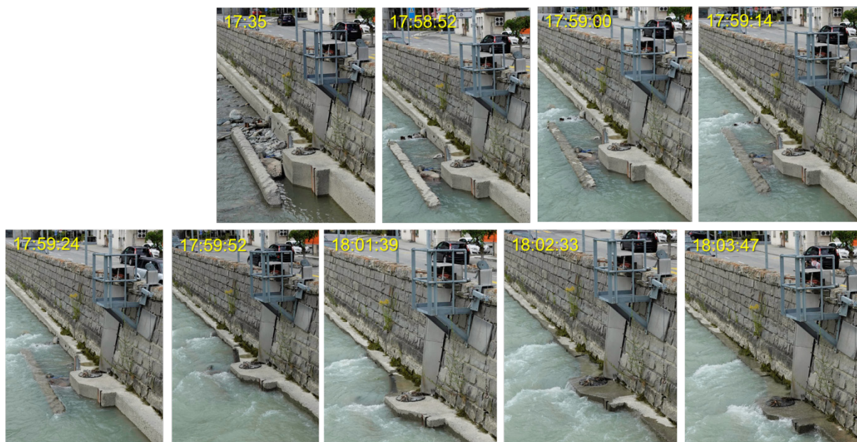
Figure 2. The same wave, attenuated downstream and with less sediment load.
